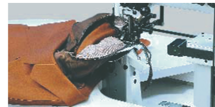
ST-697-24155操作: 把垫肩钉到袖笼上, 并切割边缘; 服装的衬里缝到袖笼上, 并切割边缘。 Operations of class ST-697-24155: Attaching shoulder pads to armholes and trimming edges; attaching body lining to armholes and trimming edges.
