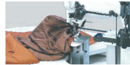
ST-697-15155操作: 嵌入式服装里袖笼缝合 Operations of class ST-697-15155: Inserting wadding strips close to the sleeve setting seam; sewing sleeve lining into armhole
